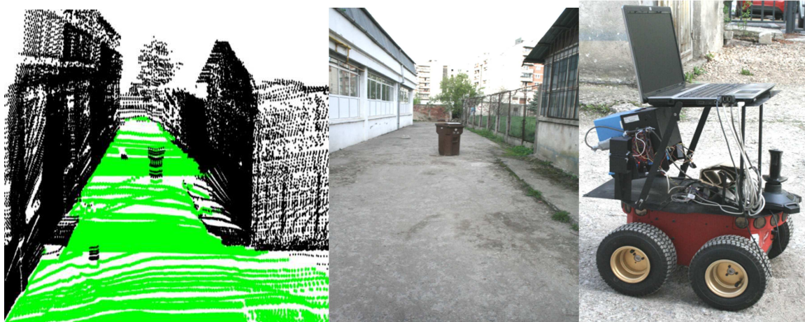
Fig. 7 A typical outdoor scan registration results; the photo of the same scenario; the custom 3D laser scanner mounted on the P3 type robot
