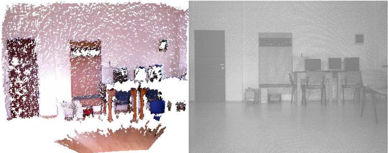
Fig. 3 Typical structural light RGB-D data and the IR image associated with the same scan from Kinect sensor
